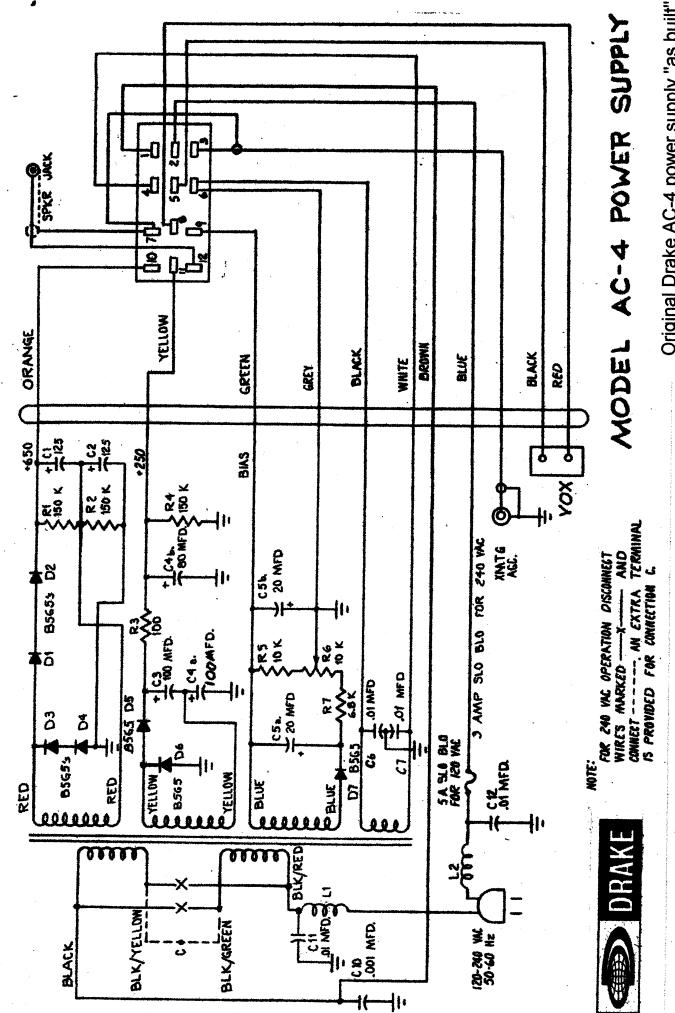
Original Drake AC-4 power supply "as built"
