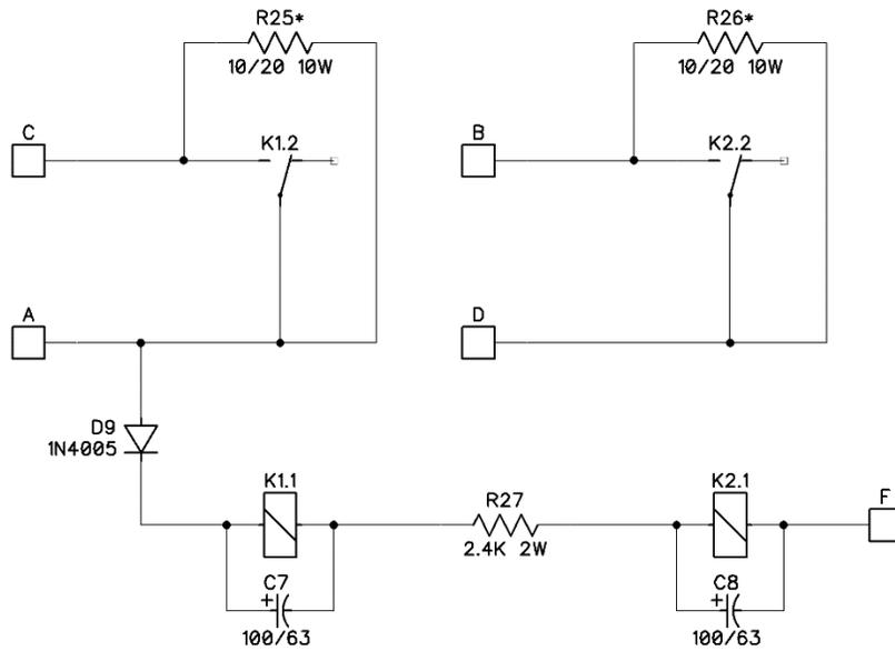
\*FOR 120VAC OPERATION, R25 & R26 ARE 10 OHM 10 WATT
