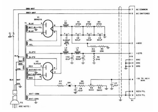
For reference, the schematic diagram of the solid-state 516F-2 power supply is shown below:
