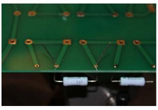
(\_) Temporarily install the completed filter capacitor PCB on the top of the chassis over the old filter capacitor mounting holes in the new mounting holes using four (4) 0.025" x 0.500" aluminum hex spacers and eight (8) #6-32 x 0.25" screws. Once the spacers are aligned remove the new filter capacitor PCB and set it aside. It will be installed after the rectifier/timer PCB is replaced.
